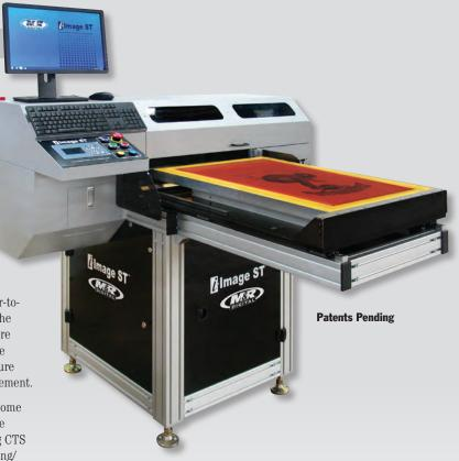
available in a single-printhead configuration. Because of their large size and capacity—maximum screen size is  $152 \times 152 \text{ cm} (60" \times 60")$  and maximum image area is  $132 \times 132 \text{ cm} (52" \times 52")$ —i-Image X and i-Image XE come standard with three industrial printheads.
