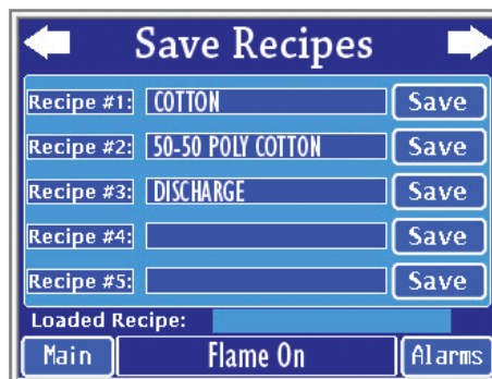
Job Recall™ allows operators to store operational parameters and recall those named settings later
