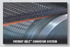
The red flexible bead stitched along one edge of the Patriot Belt™ rides in grooves machined into the large anodized aluminum SureTrak™ Rollers, providing the most precise belt tracking available (U.S. Patent Pending)
