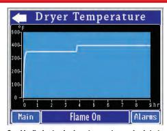
Graphic display tracks dryer temperature and substrate temperature in real time
