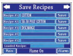
Job Recall<sup>™</sup> allows operators to store operational parameters and recall those named settings later
