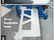
3. Mount the lightweight Tri-Loc pallet on the press. The registration pallet's three registration points precisely duplicate the registration points on the Master Registration Frame.
