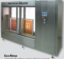
automates the tedious process of rinsing exposed screens while ensuring consistency and reducing the chance of blowing out exposed images. Balanced pressure from sprayers on both sides of the screen extends screen life. Since Eco-Rinse processes screens so quickly, per-screen labor costs can be cut by up to half. Eco-Rinse also reduces operating costs by recycling water used in the wash cycle, further lowering per-screen water usage.
