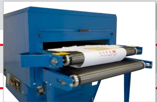
Two-belt conveyor system doubles cure time and returns garments to the load end of the dryer.
