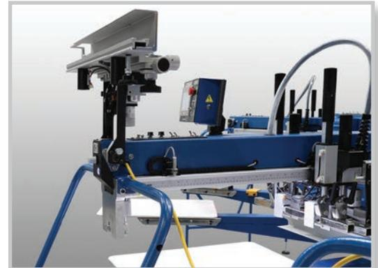
*Pneumatic-locking, Quick-Flip™ front frame holders*
