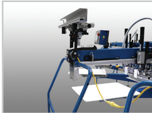
Pneumatic-locking, Quick-Flip™ front frame holders
