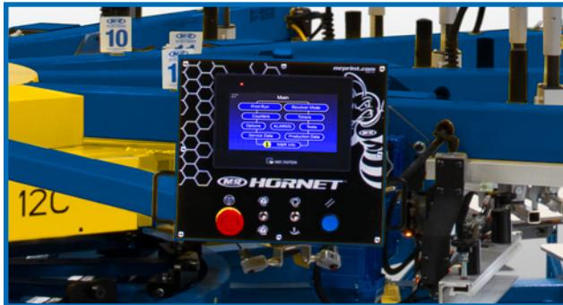
The HORNET is equipped with a 7.5-inch high-resolution touchscreen designed for fast learning and intuitive operation. A clean, modern icon system guides operators through setup and daily use with minimal training required. Integrated, multi-language tutorial screens provide step-by-step guidance directly on the display, eliminating the need to reference external manuals. This built-in intelligence streamlines onboarding and helps operators get up to speed quickly and confidently.
