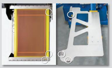
Registration points on i-Image STE, STE I & STE II precisely match the stop points on Tri-Loc pallets for blazingly fast registration
