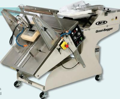
bar will retract, and the Omni-Bagger will automatically shut down and remain offline until manually reset. Engineered for dependable performance and low maintenance in demanding, high-production environments, Omni-Bagger can be easily integrated with other Amscomatic equipment to create a highly-productive folding/labeling/bagging/sealing system.
