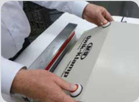
**4** Press both buttons simultaneously to engage the clamping mechanism
