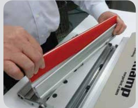
**3** Seat the squeegee blade in the opening between the two sides and place the set between the Qwik-Klamp's jaws
