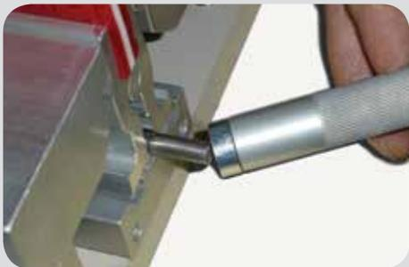
Place the set between the Qwik-Klamp jaws and press both buttons. With the clamps engaged, use the supplied magnet to remove the retaining pin. Then press either button to disengage the clamps and release the squeegee blade.
