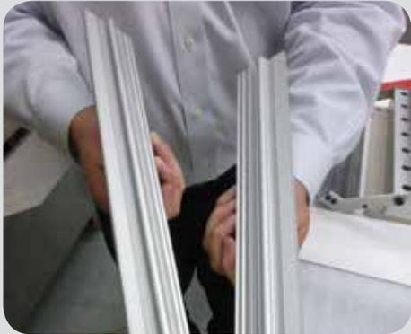
**1** Hold a bar in each hand with the interlocking sides facing each other
