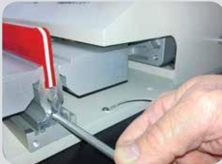
**5** Insert the retaining pin and release the clamping mechanism by pressing either button
