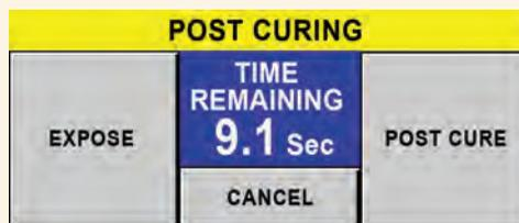
During exposure or post-curing the screen displays the exposure mode and time remaining
