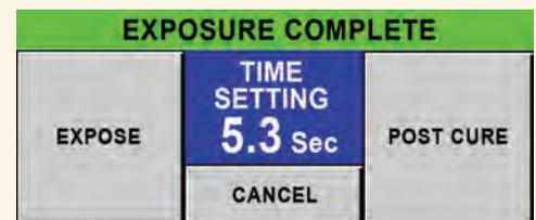
When the process is complete, the touchscreen shows EXPOSURE COMPLETE and exposure time
