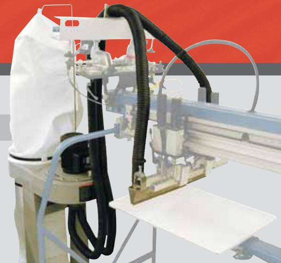
Flock-Vac is designed to remove excess flock from garments on the press. Since it eliminates up to 90% of the flock not embedded in the adhesive, Flock-Vac greatly reduces the fiber that can be drawn into the dryer circulation system. Flock-Vac mounts to any open printhead, vacuuming up loose flocking fibers as the printhead passes over the garment. Flock-Vac helps get the most out of flocking by minimizing the mess—and reducing the cleanup effort—typically associated with flocking.
