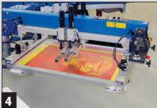
**4.** Move the registration pallet into position, pull the screen into contact with the pallet's three registration points, and lock it in place. Repeat the process for all screen frames.
