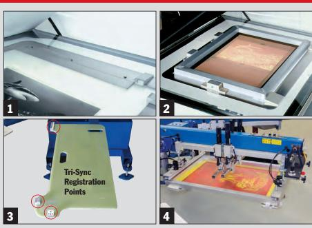
2. Insert the screen frame into the Tri-Loc Master Registration Frame. Pusher pins ensure that the screen is pushed securely up against the three registration points, and the Tri-Loc system keeps the screen and film precisely and tightly locked into position during vacuum pull-down.
