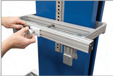
Frame holders adapt in seconds for multiple screen sizes
