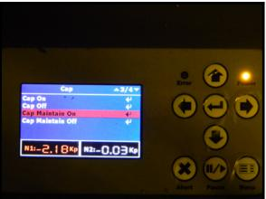
When the M-Link is capped, the print heads need to stay moist.
