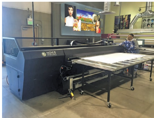
Today's grand-format printers can even tackle high-exposure jobs such as outdoor road signs. Grand format hybrids can print super-wide flexible and rigid substrates with very short change-over times. (Photos courtesy of Novus Imaging Inc.)
