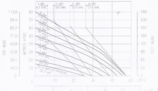
B15 Moulded Pump Performance Curve Performance based on water at ambient temperature
