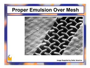
Depending on your printing application and the thickness of the mesh, the actual emulsion build-up above the mesh can be between 12 microns to well over 40 microns. For example, 110/80 mesh with a fabric thickness of 116 microns would print well with approximately 23 microns of emulsion build-up. Whereas a 230/40 mesh with a fabric thickness of 58 microns would print well with approximately 12 microns of emulsion build-up.
