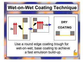
Always begin coating from the substrate side of the screen until a mirror-like glossy finish is observed from the squeegee side of the screen when viewing at a low angle to the lights. Then complete your base coating from the squeegee side.
