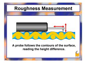
An Rz value of 15 microns means there is a deviation in surface roughness of 15 microns. The knuckles of the mesh where the threads intersect one another represents the highest point. And the open area of the mesh where the emulsion shrinks back into the weave of the mesh represents the lowest point.
