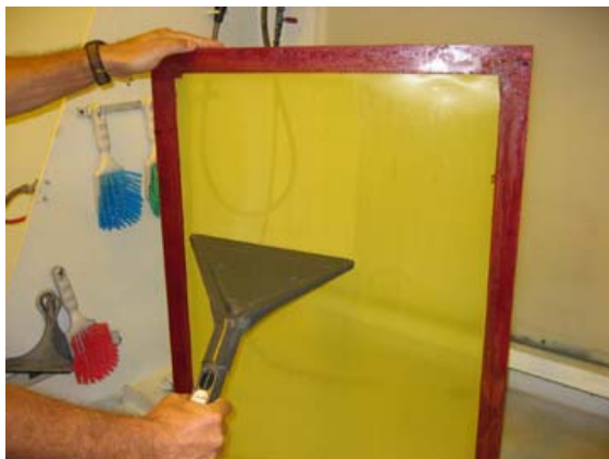
Figure 2 Water vacuum to help speed processing and reduce contamination
