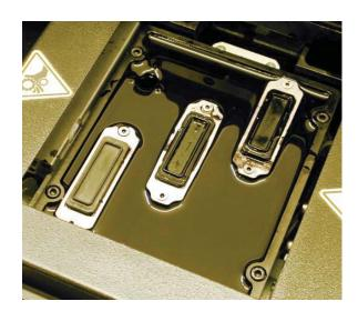
Closely inspect the capping stations for any harden ink particles or chucks, carefully wipe away any debris using caution to not damage the rubber seal.
