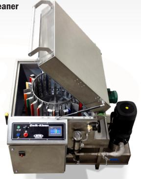
M&R's Qwik-Klean™ automates the highly labor-intensive, tedious process of cleaning squeegee holders and floodbars. Qwik-Klean achieves outstanding results through the combination of a high-volume spray and a rotating squeegee/floodbar holder assembly all within a single chamber. The addition of a final freshwater rinse eliminates the need for post-cycle washing and the possibility of squeegee degradation from chemical exposure.
